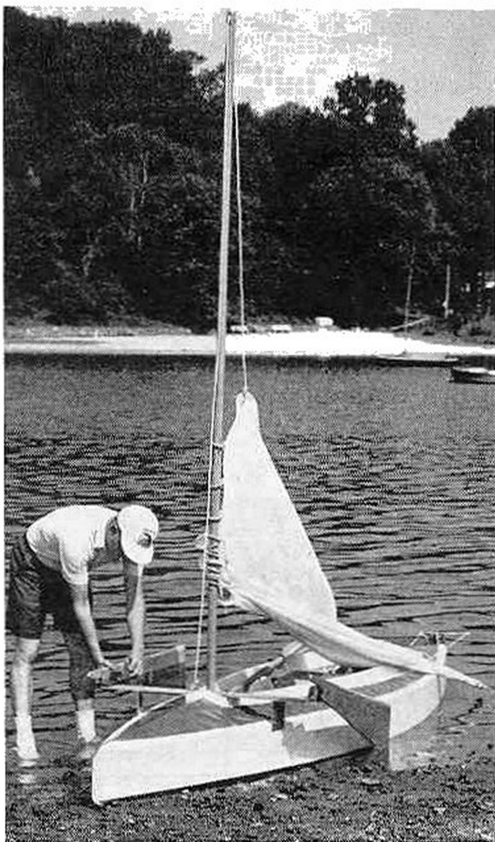
LEEBOARDS PIVOT to permit beaching boat. Wing nuts and carriage bolts lock them in "up" position
