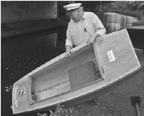
Les Brown's Micromouse Bumblebee carries its builder's 160-pound frame quite comfortably. Les modified the plans to achieve the gracefully arched decks, which provide stowage space for a collapsible cart that he uses to get his boat from his home to the water nearby. To accomplish this, he arched the tops of the transoms and used arch-topped open frames instead of square, solid bulkheads. (Les Brown)
