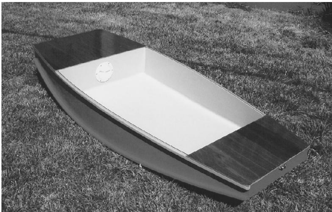
A flat-bottomed Micromouse built with external chine logs, using the simplified chine log method. (Henry Massenburg)
