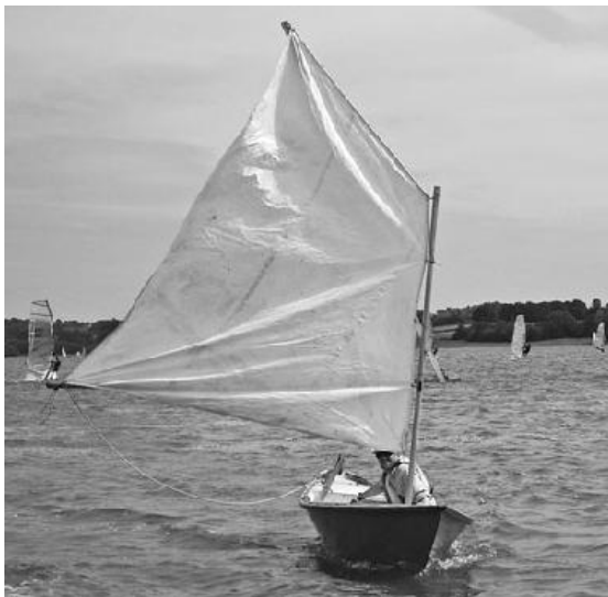
Doris the Dory isn't fast, but she is perfectly happy in conditions like this—probably around Force 5. Some people say that dories don't sail well, but with her wider-than-normal bottom and bit of ballast carried down low, Doris does just fine, even in winds a notch or two stronger than this.
