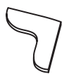
Quarter knee drawn using kitchen jars, cups, etc., and then cut out
