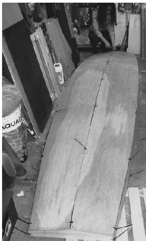
Nylon cable ties are used to “stitch” together the hull panels of Anthony Smith’s Cruising Mouse. Since you’ll be fiberglass-taping the inside of the hull first, place the clasps of the cable ties on the outside of the hull. (Anthony Smith)
