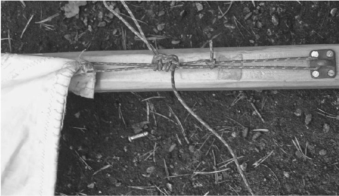
The same temporary bight used at the tack (bottom of the sail nearest the mast) to tighten the luff of the sail.
