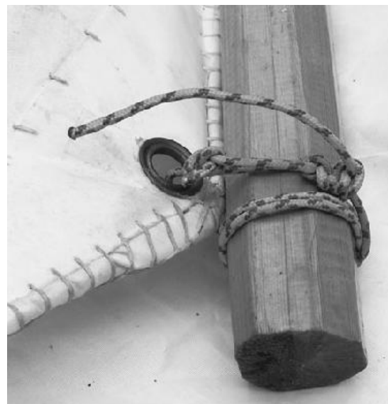
Tying the temporary bight used to attach the head of the sail to the mast.
