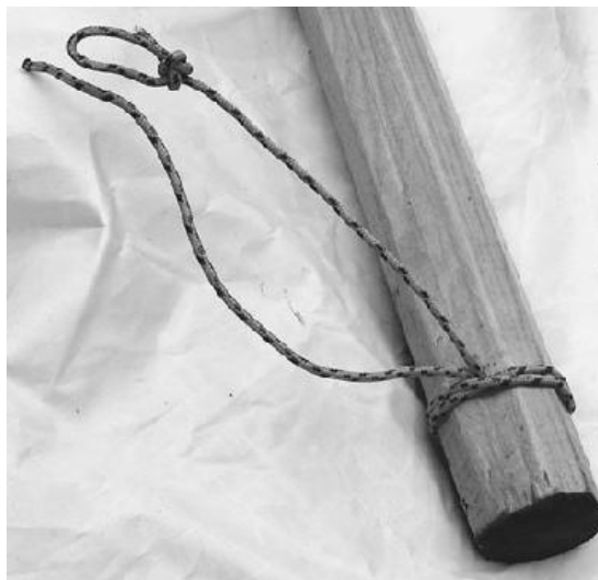
The lashing at the top of the mast goes around the mast a couple of times to prevent stresses that could cause the mast to crack. One end has a bowline tied in it.
