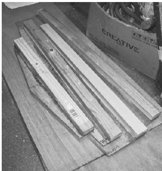
These transoms and bulkhead frames all have their top cleats glued in place flush to the top edge of the plywood. For chine log construction, additional cleats would be added to the bottoms and sides. (Anthony Smith)
