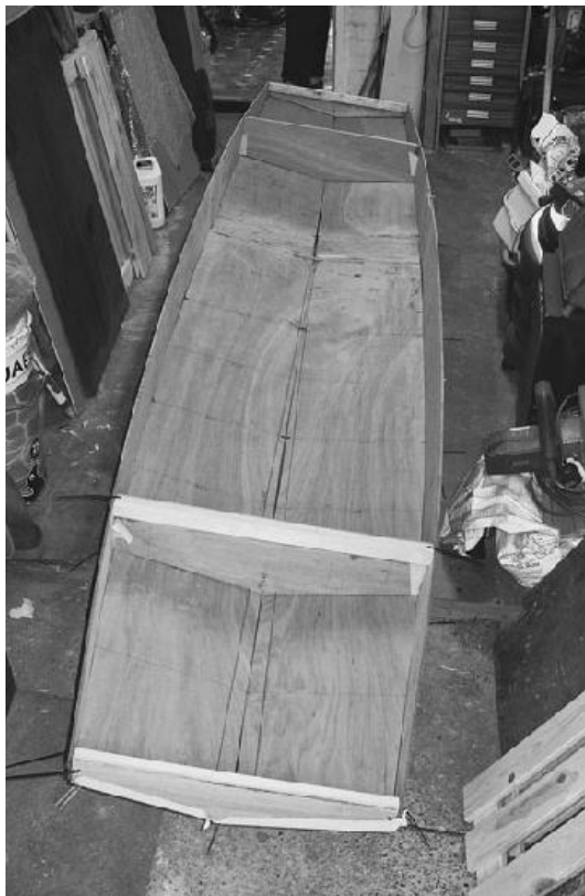
Nylon cable ties are used to “stitch” together the hull panels of Anthony Smith’s Cruising Mouse. Since you’ll be fiberglass-taping the inside of the hull first, place the clasps of the cable ties on the outside of the hull. (Anthony Smith)
