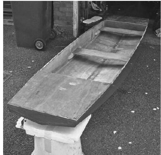
Raising your work off the floor will make construction and painting easier. If good sawhorses aren't available, you can make do with a kitchen table, a pair of 5-gallon pails, or almost anything that's stable and strong enough. Anthony Smith put together some homemade stands using expanded polystyrene for the purposes of painting his boat. (Anthony Smith)
