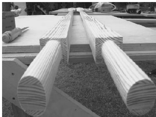
A pair of laminated oars under construction, showing the taper of the blades. The handles or grips should be round when finished. (Ben Crawshaw)
