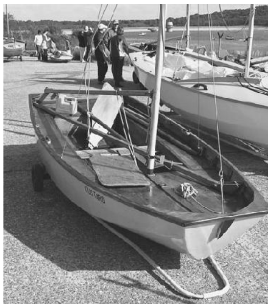
Designed by Jack Holt and Barry Bucknell, the Mirror sailing dinghy was the first dinghy to be built in any numbers using the stitch-and-glue method, although canoes had previously been built using the technique. It's still a popular boat, and kits, hulls, and parts can be obtained from Trident in the United Kingdom at www.trident-uk.com .
