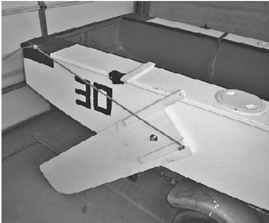
The leeboard arrangement Shorty used could not have been much simpler either.
