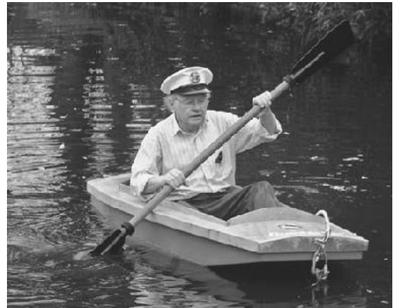
Les Brown's Micromouse Bumblebee carries its builder's 160-pound frame quite comfortably. Les modified the plans to achieve the gracefully arched decks, which provide stowage space for a collapsible cart that he uses to get his boat from his home to the water nearby. To accomplish this, he arched the tops of the transoms and used arch-topped open frames instead of square, solid bulkheads. (Les Brown)
