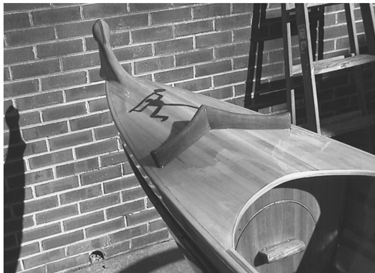
FIGURE 6-25. Kent Robertson's Ulua with a traditional Hawaiian manu and splash guard. (Photo courtesy Kent Robertson)
