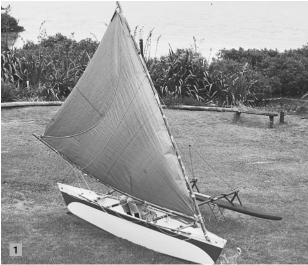
FIGURE 12-6. Oceanic lateen rig close-hauled on a port tack.
