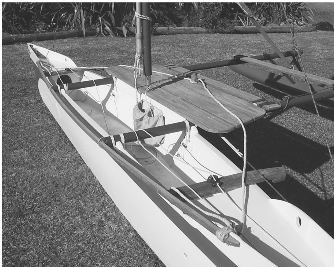
FIGURE 10-20. A windward-side hiking seat on the T2, with a wooden knob bolted in place to snub the sheet. Note the leeward side guide rail to aid in shunting an Oceanic lateen sail.
