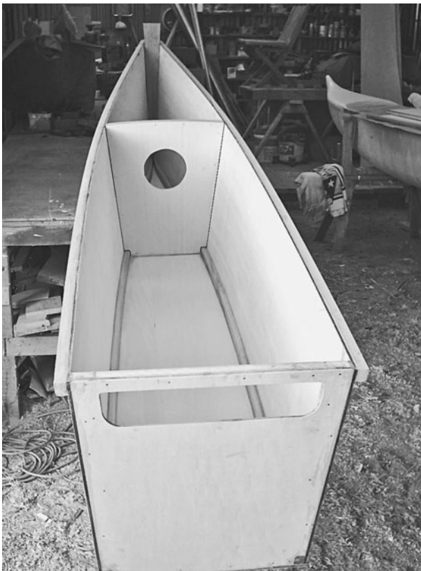
FIGURE 7-11. Hull section with bottom panel installed.
