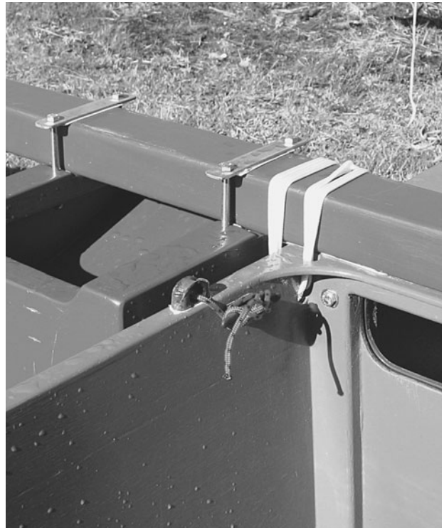
FIGURE 10-17. The Wa'apa's outboard bracket is mounted below the iako with four \frac{5}{16} " (8mm) bolts.
