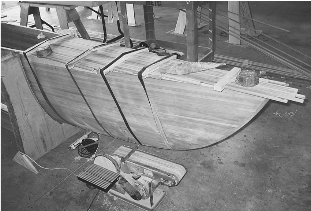
Figure 6-23. T2 deck being glued to the hull. (Photo courtesy Clay Ghylin)
