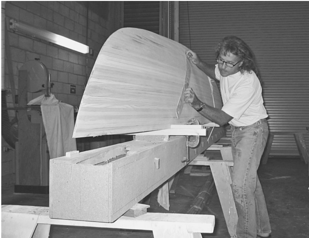
FIGURE 6-20. Fairing a T2 hull before glassing. (Photo courtesy Clay Ghylin)
