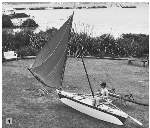
FIGURE 12-9. The tack line is secured in a cam cleat when the yard reaches the new bow.
