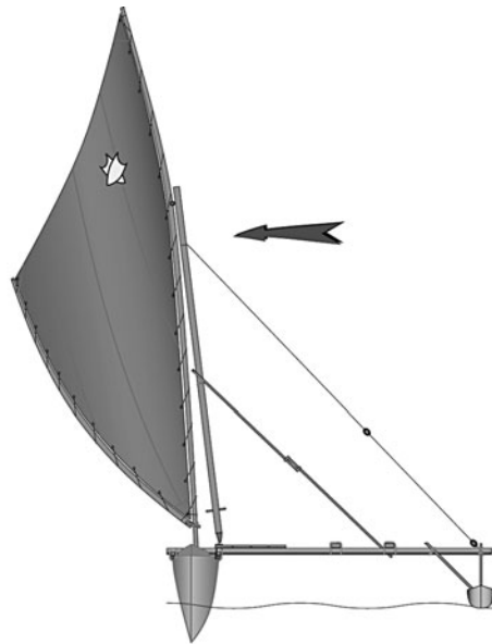
In light winds the mast is eased to vertical or to leeward.
