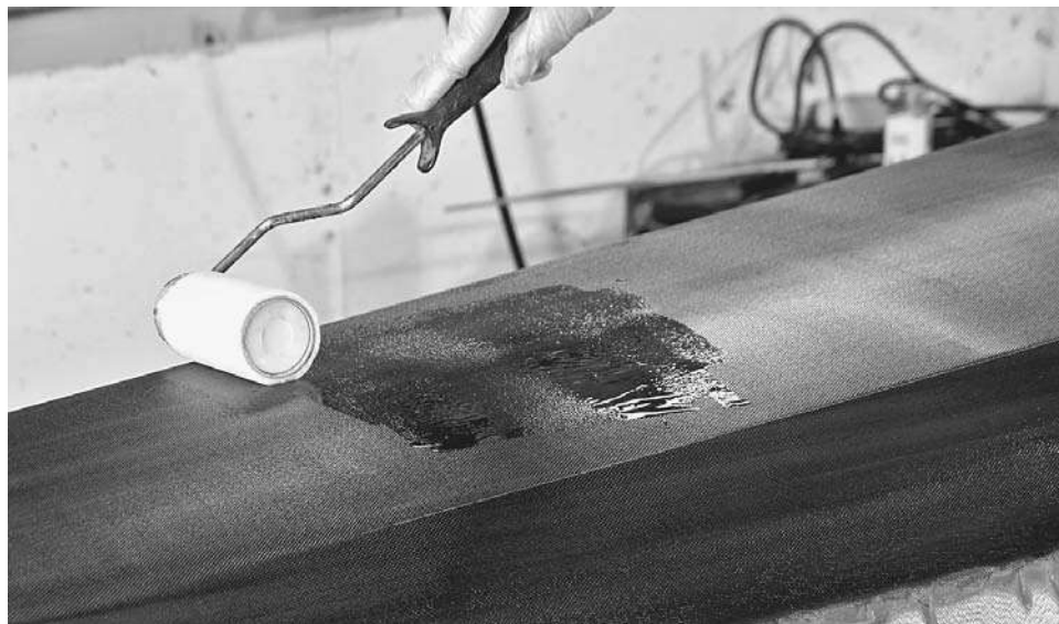
Figure 13-47. You can build up the fill coat slowly using a roller to add multiple, thin coats. On this boat I am going to apply another complete layer of glass across the hull and up onto the deck, after joining them together. Because of this I do not want to apply a fill coat that completely fills up the weave texture. This would result in a thick layer of epoxy between the layers, which would add weight but not much strength. I do, however, want to fill up the weave enough at this time so that it does not trap crud before I'm ready to apply the second layer of glass. Rolling on a moderately light coat will get the job done for now.
