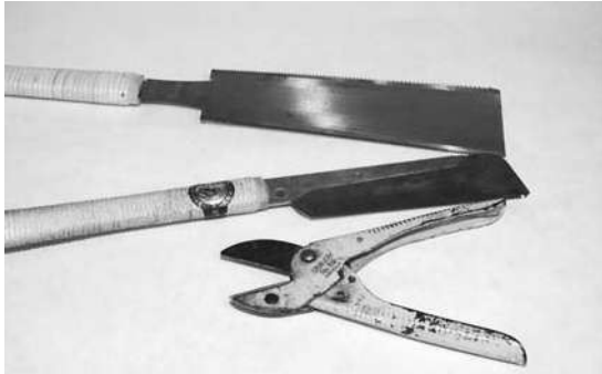
Figure 3-8. Cutting strips to length can be done with a saw or shrubbery pruners. Shown here are Japanese-style pull saws, which cut on the pull stroke, allowing a very thin blade that cuts very quickly and easily. The top saw has both a ripping blade and a cross-cut blade.
