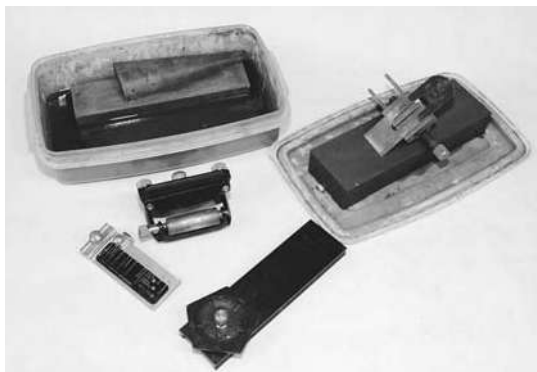
Figure 3-1. Sharp tools make just about everything quicker, easier, and more precise. You can do a good job sharpening your tools with sandpaper stuck to a piece of glass, or use waterstones as shown. The little jig that holds the plane blade on the right will shorten the time spent sharpening, or you can use the more sophisticated jigs shown below the stones.
