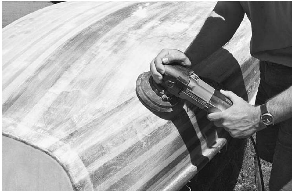
Figure 11-38. The fill coat should leave a quite smooth surface, but a good finish often requires some serious sanding. Start with 60-grit sandpaper on your random orbit sander. On the boat shown there were some rough spots along the edge where the fiberglass doubled up. The goal is to feather in these edges and level any irregularities in the surface so there are no shiny spots left on the surface. Along the edges of additional layers you will need to sand into the glass a little bit. However, if you start seeing signs of the fiberglass showing up elsewhere in the surface immediately adjacent to shiny spots, stop sanding that area. You will need to add another fill coat.
