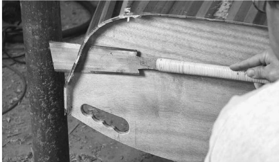
Figure 11-22. Trim the ends of the strips even with the transom. A Japanese pull saw does a good job trimming quite flush, but it is possible to get out of alignment and scar the transom. Be careful that the blade is not scratching up the transom as you cut. Round over the corner with a block plane and sand it to prepare for fibreglassing.
