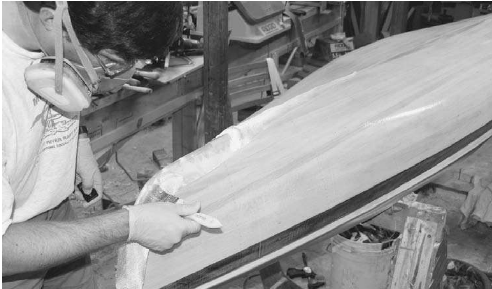
Figure 12-36. Cover the stem with at least one layer of bias-cut fiberglass. Extend this cloth down the centerline for extra abrasion protection.
