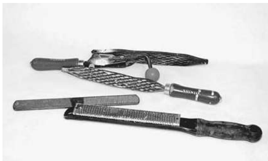
Figure 3-7. Files, rasps, and microplanes can deal with tricky wood that may aggravate a plane. Shinto wood rasps will quickly remove wood or delicately remove epoxy sags. The 4-in-Hand on the left will do the same or soften a sharp edge of fiberglass. The microplane at the bottom has many tiny blades that shape wood easily.
