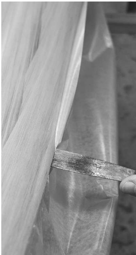
Figure 13-43. Slide a sheet of waxed paper in between the deck and hull to protect the other half as you stain and epoxy. The seam may be quite tight—I find that a putty knife helps coax the paper into the sheer seam.
