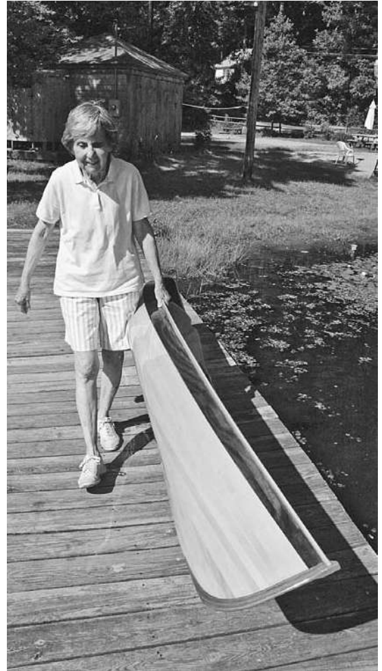
Figure 12-39. The finished Nymph is a cute little boat suitable for exploring small lakes and ponds with a minimum of fuss. It is light enough to carry with one hand, but it is still quite rugged.
