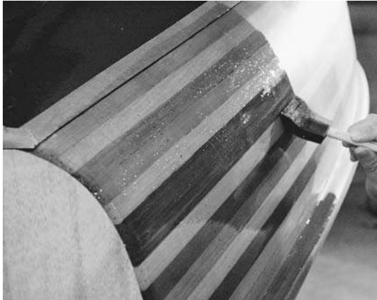
Figure 10-11. After the varnish is on the section, even out the coat with vertical strokes. Use moderate pressure to pick up varnish from thick areas and move it to sparse areas. Do not redip the brush. Look for holidays where there is no varnish by putting your eye close to the surface and looking toward the light.
