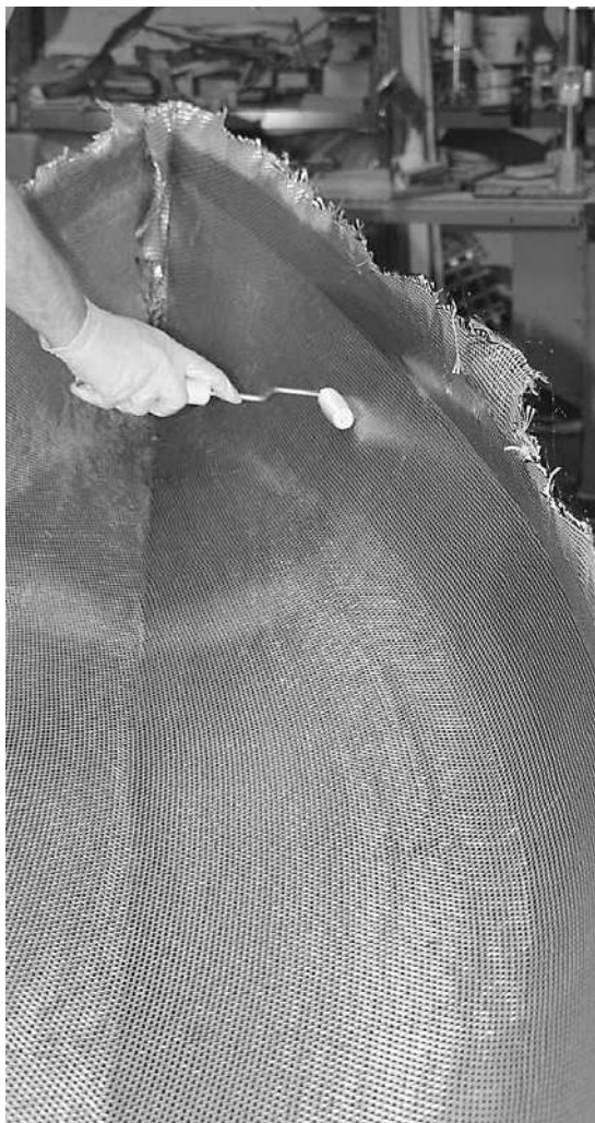
Figure 12-26. A bubble roller (a grooved roller tool intended for removing bubbles from fiberglass) helps press down the cloth tight against the wood, driving any excess resin under the cloth up to the surface. While not really useful with light fiberglass, the roller can help create a lighter layup with this thicker hybrid cloth.
