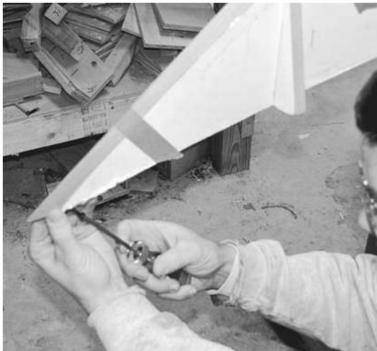
Figure 5-30. Secure the inner stem with tape and maybe a screw. Make sure the screw is accessible so it can be removed. Remove the tape before stripping over it.
