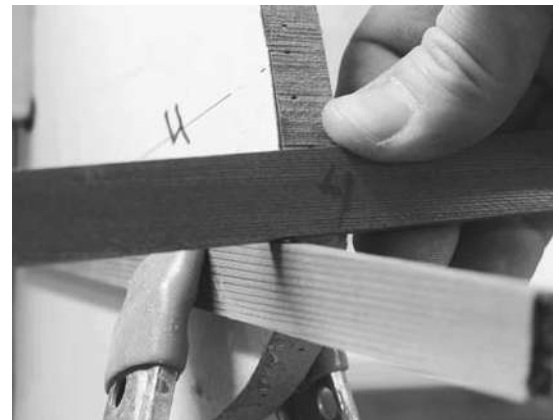
Figure 6-5. The first strip, or sheer strip, of a closed boat such as a kayak is just one situation where you may need to create a rolling bevel. The goal is to create a tight seam on the outside of the hull. Marking each form number onto the strip at the point where they intersect will make it easier to find your spot as you plane the bevel. As you press the strip against the clamped-on scrap, notice the size of the gap between the strip and the scrap. This is how much you need to bevel the strip. If you are fitting against an existing strip, you will again want to note the size of the gap. While you are looking at one form, also look at the forms before and after this one and note the differences in the bevel at each form.
