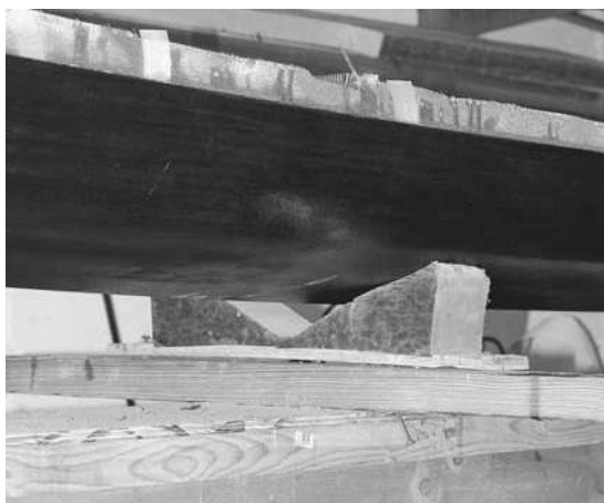
Figure 9-22. I use some V-blocks made of foam to hold the boat after I flip it over to work on the inside. You could also cover some blocks of wood with carpet scraps or make slings to support the boat.
