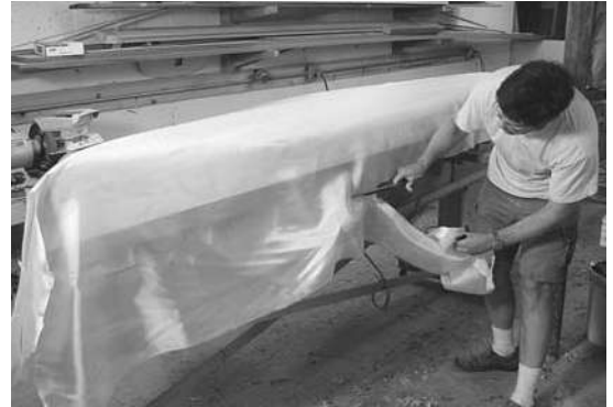
Figure 9-8. A little fiberglass hanging below the boat absorbs drips and keeps them off the floor, but this can also waste some perfectly good cloth. I trim the edge several inches below the sheer/gunwale.
