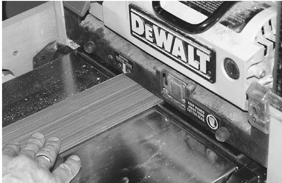
Figure 5-9. Using a consistent thickness of strips helps produce a smooth surface, but this is particularly important with cove-and-bead strips. It is almost impossible to keep the cove-and-bead centered on the strip if the thickness varies. Running the strips through a thickness planer after they come off the saw solves the problem. Here I'm running five strips through simultaneously.
