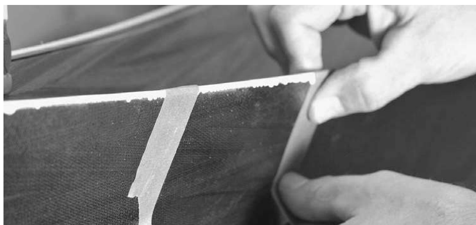
Figure 13-48. I installed a feature strip of light-colored contrasting wood along the top edge of the hull after the rest of the outside had been stained and fiberglassed. I glued it down and secured it with tape. After installation you can glass the inside. The outside will be reinforced when the deck is attached and the seam is glassed.
