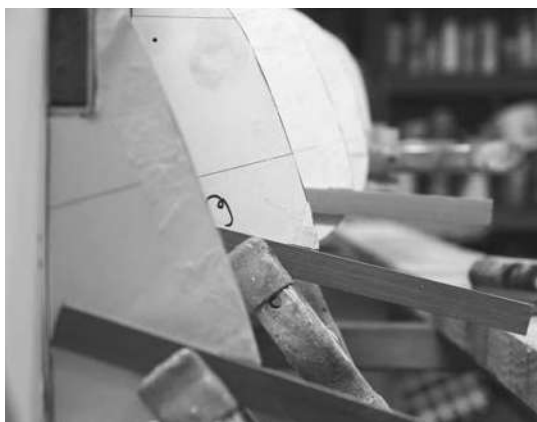
Figure 13-18. A closed boat like a kayak may have a constantly changing bevel between the deck and hull. This rolling bevel is indicated by temporarily clamping scrap strips at the sheerline so that they bisect the angle between the deck and hull. Use these scraps as guidance for planing the bevel on the first sheer strip, that is, the topmost strip on the sides of the hull.
