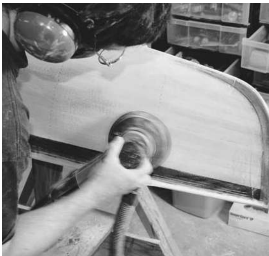
Figure 10-6. Where you have extra layers of glass, such as around the stem, you will need to feather in the edge of the glass. This will require sanding into the glass of the thicker layer and blending it down to the surface of the surrounding glass.
