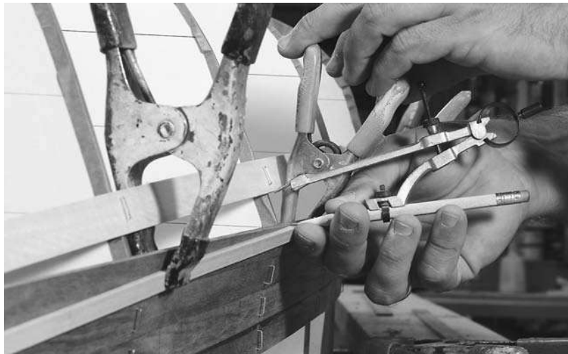
Figure 12-15. Staple a strip on the mark you just made and check that it is fair. Then use your compass again to adjust the location of another strip clamped to the installed strips. When this strip is smooth and fair, mark a pencil line along the top edge of this strip. This indicates where you will trim the excess off the existing strips. A Japanese pull saw does a good job cutting off the excess. Cut a little above the line.
