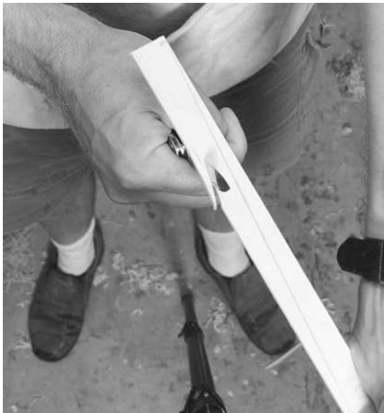
Figure 6-22. A jackknife quickly removes excess wood as you taper the end of a strip. When you get as close as comfortable with the knife, switch to a block plane.
