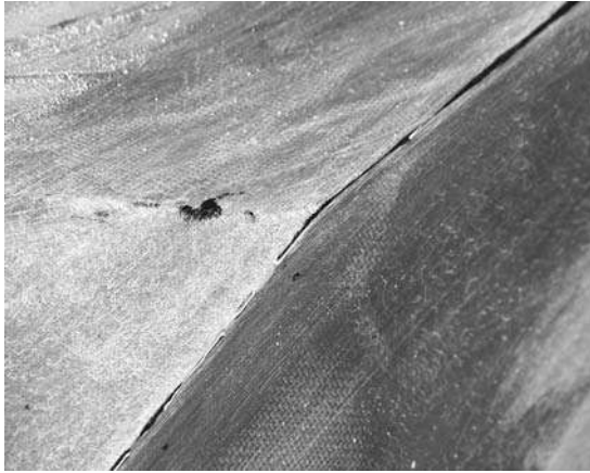
Figure 10-5. It is extremely easy to sand through sharp edges and feature lines. Avoid touching these corners with a power sander. You would likely go through the material before you can blink. Instead, keep the pad of the sander flat on the large surfaces, leaving the corners shiny until you are done with all the power sanding, then hand sand with fine sandpaper to lightly remove the gloss.
