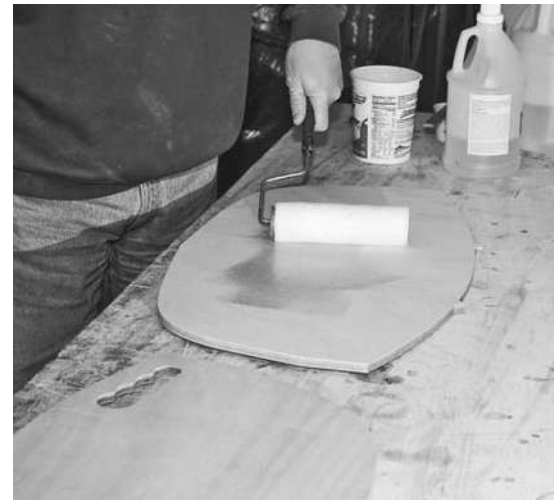
Figure 5-31. Any plywood parts such as transoms that will remain in the boat after stripping should be coated with epoxy to protect the wood from glue drips and other damage.
