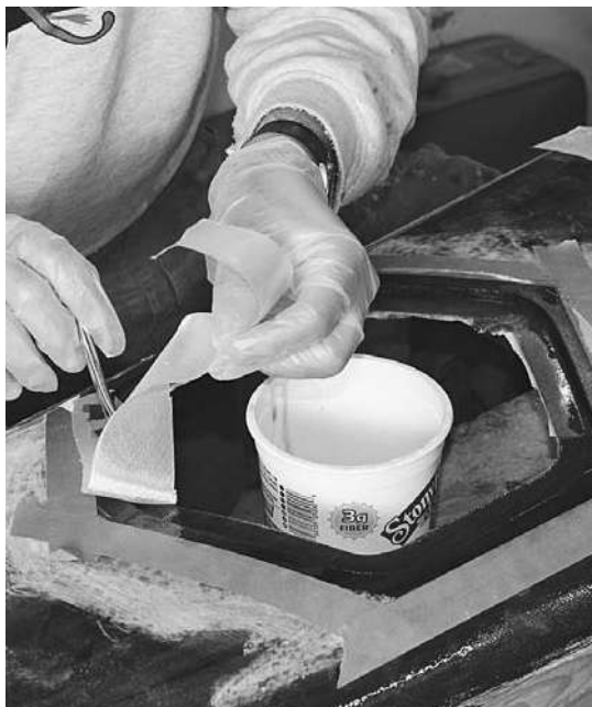
Figure 13-62. The hatches need a spacer between the lip and the deck to allow for a gasket. The spacer is set in epoxy thickened with colloidal silica to make a mayonnaise-like glue. Try to clean up any squeeze-out while the glue is still wet. After the glue has set, clean up the inside edge of the hole.
