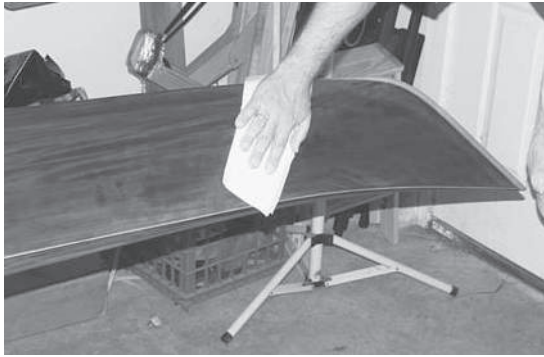
Figure 10-8. Remove dust from the surface of the boat before varnishing by vacuuming, rinsing it with water, and then wiping with a tack cloth.
