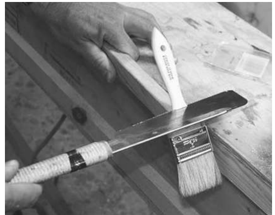
Figure 9-34 Unless you have really long arms, you will need a special tools to access the far reaches of the deck/hull seam—enter “brush-on-a-stick.” Screw a chip brush to the end of a 1-inch by 1-inch by about 8-foot stick, and then saw off the brush handle.
