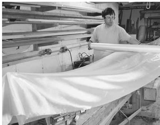
Figure 9-6. It does help to have an assistant when rolling out the fiberglass. Working alone it is easy to snag something, and even the pressure of rolling the cloth on the boat surface can distort the fabric a little bit. But with care and a pair of scissors in your pocket before you start, you should be able to handle the task alone. Note that the waxed paper is still in place between the deck and the hull.
