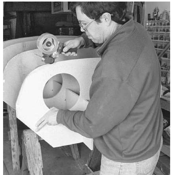
Figure 5-25. Wrap tape around the edges of the forms to keep glue from sticking. This clear packaging tape will assure nothing sticks at all. Masking tape also works well. It allows the glue to help hold the strips to the forms a little bit, but it still lets the glue break free when needed.
