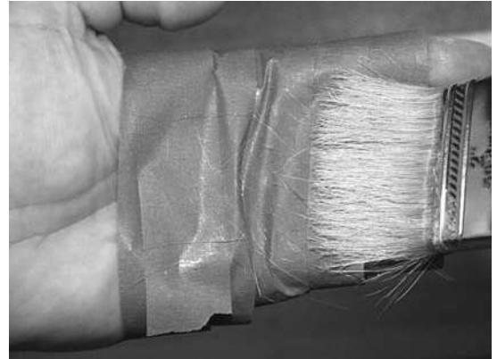
Figure 9-29. Most of the bristles that are still loose after gluing can be removed by vigorously wiping the brush against tape wrapped around your hand with the sticky side out. You may find an occasional stray hair as you paint epoxy on the boat that you can lift off with the tip of your brush.
