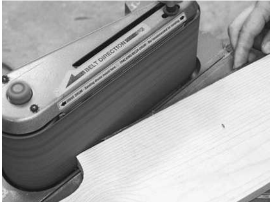
Figure 6-2. You rarely need to make one continuous strip out of two strips that will hold together on their own, but when you do, a scarf is the way to do it. Scarfs are long, tapered joints that supply a lot of glue area; this gradually distributes any load between the two ends. You could plane the taper onto each strip, but a simpler method is to set up a fence against a belt sander. Slide the strip along the fence until you have a sharp end. Repeat for the other strip to make a matching taper.
