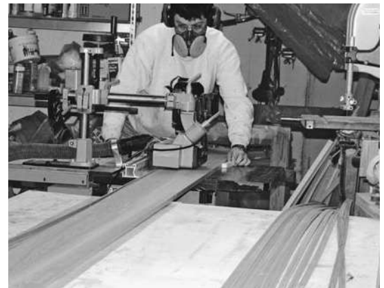
Figure 5-3. If you are cutting a lot of strips, a power stock feeder is a nice luxury. It feeds the board at a constant rate while holding it down on the table and firmly against the fence all while keeping fingers away from the spinning blade. Notice I am wearing ear, eye, and breathing protection while making all that noise and dust.
