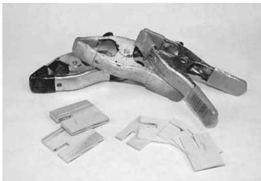
Figure 3-11. To temporarily hold the strips in place, you can clamp little U-shaped jigs that fit over the strips to the forms.
