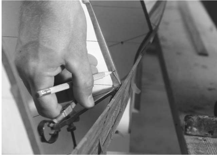
Figure 12-14. When preparing to mark the edge of the tumblehome area, make a mark a uniform distance from the tumblehome diagonal with a compass.
