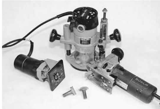
Figure 3-13. Some other useful power tools include routers and jigsaws. The large router in the middle is mounted in a plunge frame that can be used to make some specialty parts. Mounted to a table it can be used to mill cove-and-bead strips with the cutter bits shown below. The trim router on the left is useful for rounding over gunwales. The jigsaw on the right does a good job cutting hatches.
