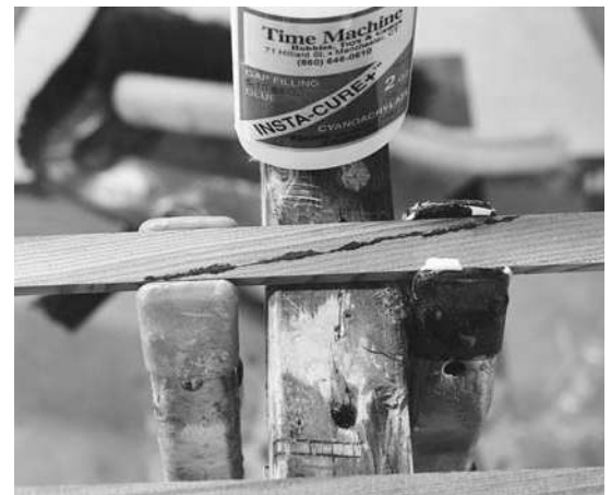
Figure 5-8. Every once in a while mistakes happen. This strip broke along the grain. Throwing the strip out would have messed up the book matching pattern. Instead, I used some CA glue to put it back together. Under fiberglass no strength will be lost, and the repair will disappear.
