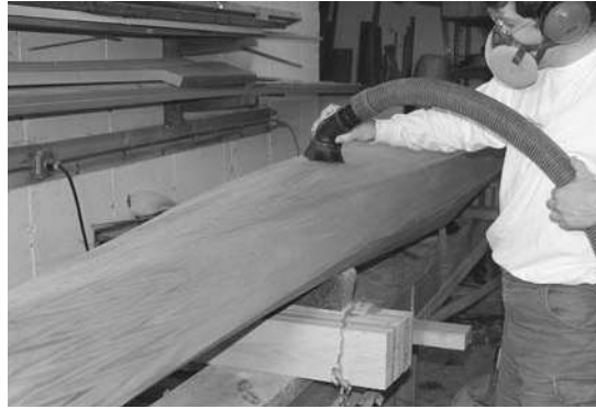
Figure 7-14. Sandpaper leaves a little bit of grit behind that will continue to scratch the boat when you switch to a finer paper. Vacuuming the boat between grits may help you get a better finish. A final vacuuming of any residual sanding dust when you are done will give a cleaner look to the final finish.
