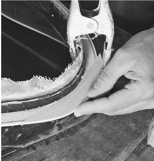
Figure 13-54. Since the laminations are not completely around the front of the cockpit, you need to finish off the front. Trim the ends of the lamination at a tangential angle with the coaming riser, creating a smooth curve across the front. Cut a piece of \frac{3}{16} -inch-thick curly maple to fit across (you could also laminate pieces instead).
