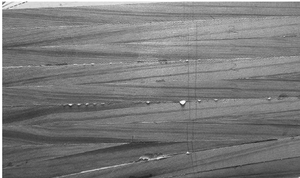
Figure 13-25. When book-matching strips you may want the grain to align across the whole face of the surface. The double line in this image was drawn across all the strips while they were aligned side by side on a workbench. Then they were fit together on the boat using these lines as alignment marks. This example uses an alternating book-matching scheme.
