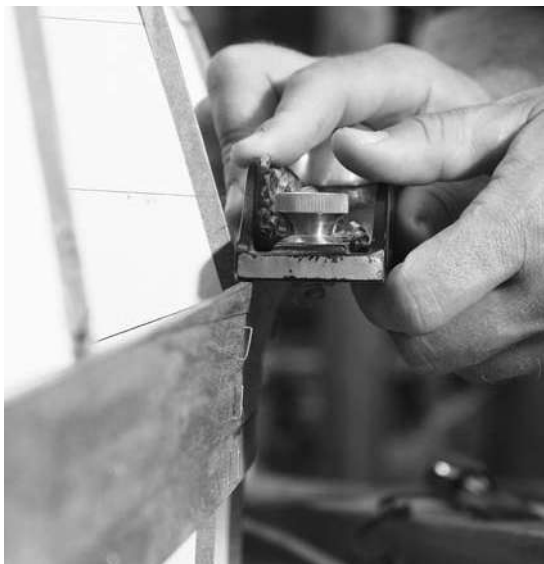
Figure 12-16. Clean up the edge with a rabbet plane. Try for a smooth, fair curve with a consistent angle on the bevel.
