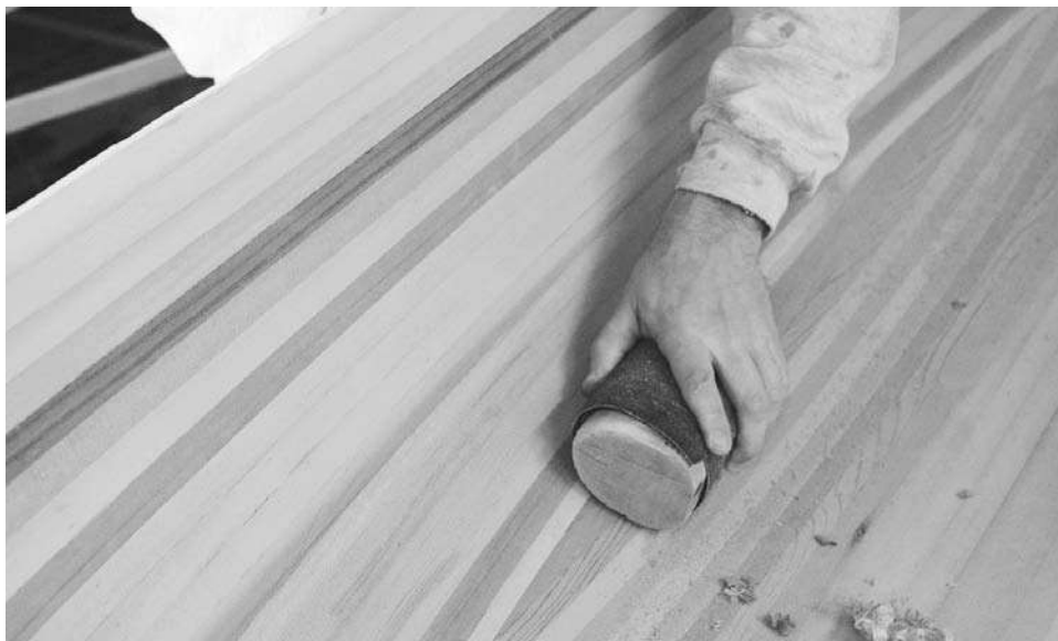
Figure 11-25. After scraping off any glue drips with a paint scraper, use a piece of coarse sandpaper wrapped around a piece of shaped foam or wood to start smoothing the inside.
