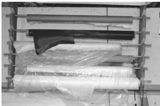
Figure 2-4. To help keep the fabric clean and undistorted, make a fabric dispensing rack from 2 by 6 lumber and electrical conduit to hold the rolls. Shown on this rack are black carbon fiber cloth, Kevlar (straw colored), and some different kinds of fiberglass. The plastic keeps dust off the material.
