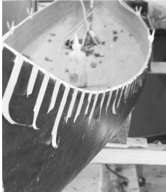
Figure 8-2. Staining some of the wood stains all of it. If you want an accent strip, it may be easiest to add it after the wood has been stained. Here the outside of the hull has been stained and fibreglassed. I'm applying a thin strip of wood to the top edge, and then I'll glass the inside. I'll glass the outside when I attach the deck.
