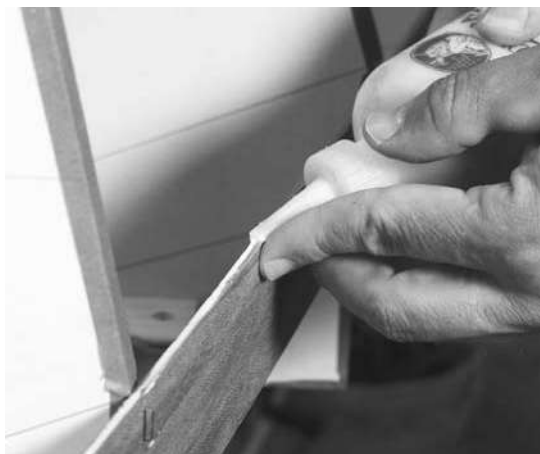
Figure 12-13. It doesn't take a lot of glue to secure the \frac{1}{8} -inch-thick strips in place, but it can be hard to direct it onto the narrow edge. It pays to have a fairly small hole in your glue dispenser so you don't get big drips coming out everywhere. With cove-and-bead strips it is quite easy to run the tip of the glue bottle down in the cove, but if you are applying glue to the bead or on a square-edged strip, you may find it helps to hold the bottle with your finger against the tip as a guide to run along the side of the strip.
