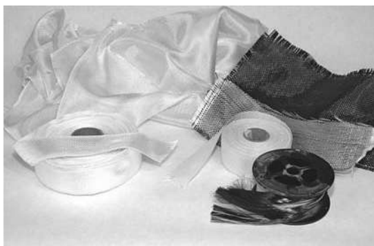
Figure 2-5. Reinforcing fabrics are available in a variety of materials. The white fabrics on the left are fiberglass, which becomes clear when saturated with resin. The black carbon fiber (top right) stays black. Woven tapes of different widths (middle right) are available for reinforcing and joining parts. The spool on the lower right contains carbon fiber “tow,” an unspun roll of fibers that can be used to make reinforcing ribs.
