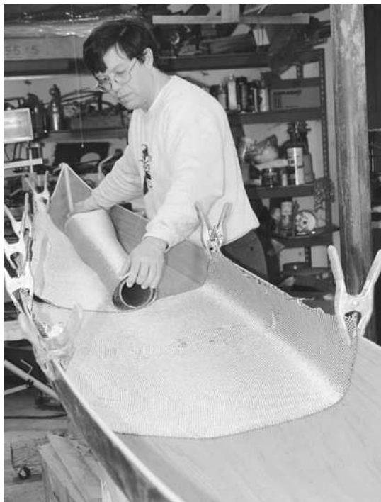
Figure 9-7. The most efficient way to cut the cloth is to lay it across the boat, overlapping adjacent pieces by about 1 inch. This is not as desirable on the outside because the overlaps create bumps running across the boat, but on the inside it works very well with minimum waste of fabric.
