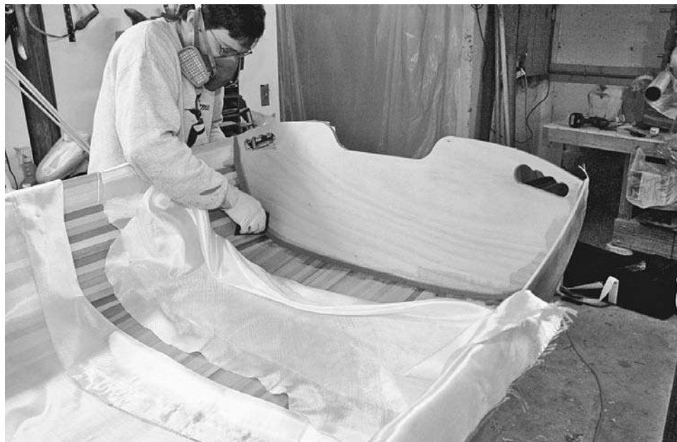
Figure 11-26. The transoms need a fillet to help the glass conform to the shape and to add strength. Use a ziplock bag to pipe in dookie schmutz, then press it in with a spoon and clean up the excess.
