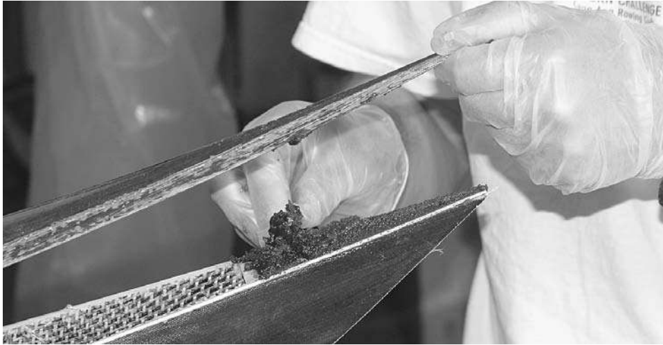
Figure 13-67. With a premade end-pour you need to secure the deck to the pour when you first start joining the deck to the hull. Spread enough thickened epoxy on the pour to securely glue down the deck. Carefully align the deck before taping it down with strapping tape.
