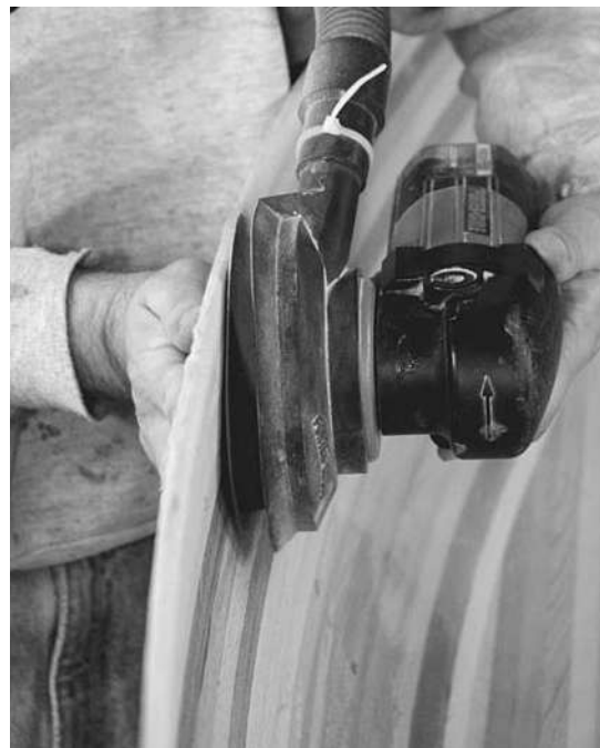
Figure 7-12. A soft contour pad on the sander helps conform to the surfaces. While working on the inside, support the sides of the boat with your hand as you sand. Hook up the sander to a vacuum cleaner to control the dust.
