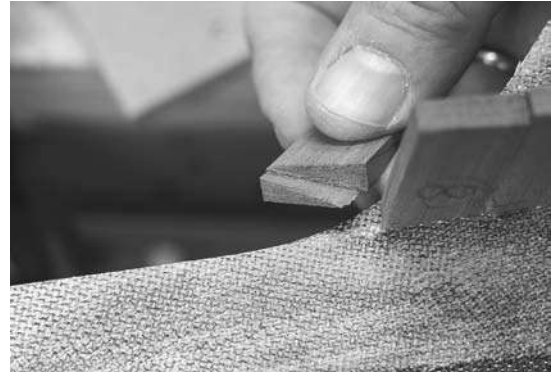
Figure 13-50. The cockpit has a coaming around the hole. Start at the front and back of the coaming and glue a series of strips vertically into the hole to create the vertical part, or riser. Proceed down each side. You can't glue the strips to the edge of the hole in the thigh brace area, so instead glue their ends and stand them up in place. While this is not strong at the moment, once it is all fiberglassed, it will be plenty tough. At the transition at the end of the thigh brace, the strips change from being end-glued on top of the deck to being side-glued to the edge of the hole. Use a utility knife to carve the end. Proceed around the full circumference of the cockpit. Use hot-melt glue to hold everything in place until the fiberglass and epoxy are applied. Use a wedge-shaped strip to close up the final gap.
