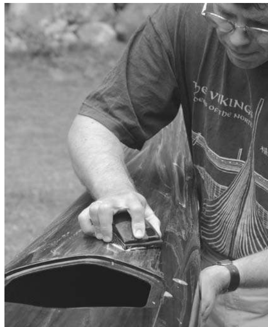
Figure 10-14. Between coats of varnish you can either wet sand by hand or use fine sandpaper in a power sander. This levels the surface and helps you see your new coat of varnish by dulling the surface.
