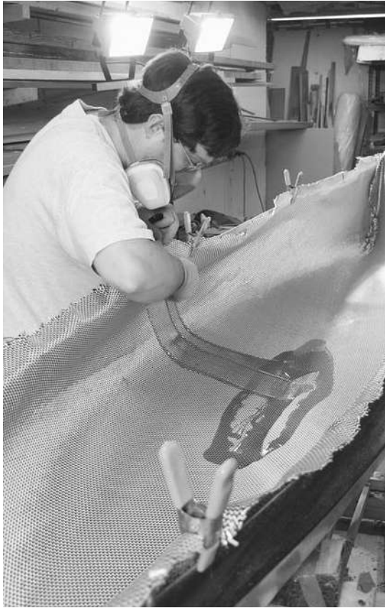
Figure 9-13. On the inside, start by dumping epoxy in a nice puddle in the middle of the boat, then pull resin up the sides with a squeegee.
