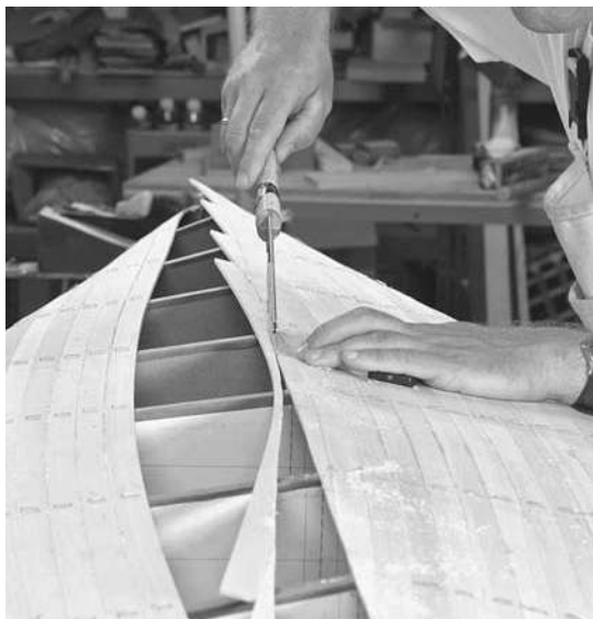
Figure 12-17. Using a similar method as you used for the tumblehome edge, mark the centerline of the strip, cut off the excess, and plane it straight.
