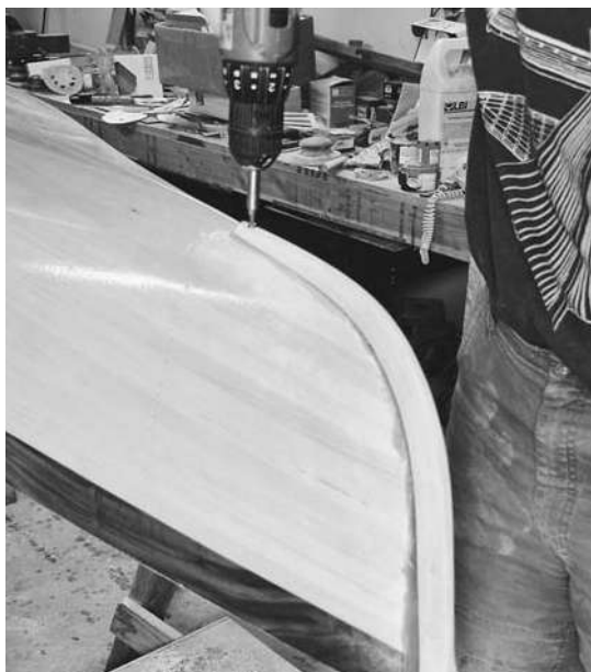
Figure 12-28. It will help if you do some preliminary shaping before installing the stem. Butter up the mounting surfaces with dookie schmutz. A screw at each end of the stem should be enough to clamp it in place. Clean off the squeeze-out before it hardens.
