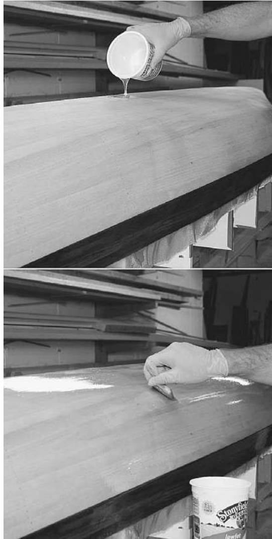
Figure 12-24. Surfboard shapers use the hot-coat technique to apply a fill coat to the fiberglass. This involves dumping a big puddle of epoxy and quickly spreading it around with a brush. On a small boat like this, where you can keep up with the drips, this system actually works pretty well. If you are a little timid about getting a big puddle of epoxy on your floor, you may want to use the more controlled method of painting on a fill coat. When the epoxy has cured, trim off the excess fiberglass with a utility knife and remove the screws holding the forms to the strongback.
