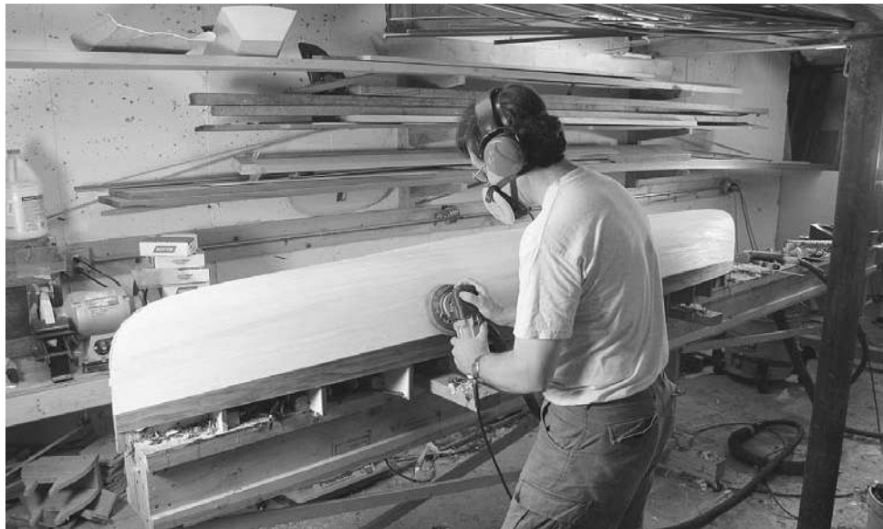
Figure 12-22. Start with coarse sandpaper in a random orbit sander to smooth the surface. Progress up through finer-grit sandpapers, finishing with 220. With hardwoods, you will want to go to finer sandpapers than with softwoods, as they tend to show scratches more readily. Be sure to keep replacing the sandpaper as it gets dull so you aren't just burnishing the surface.
