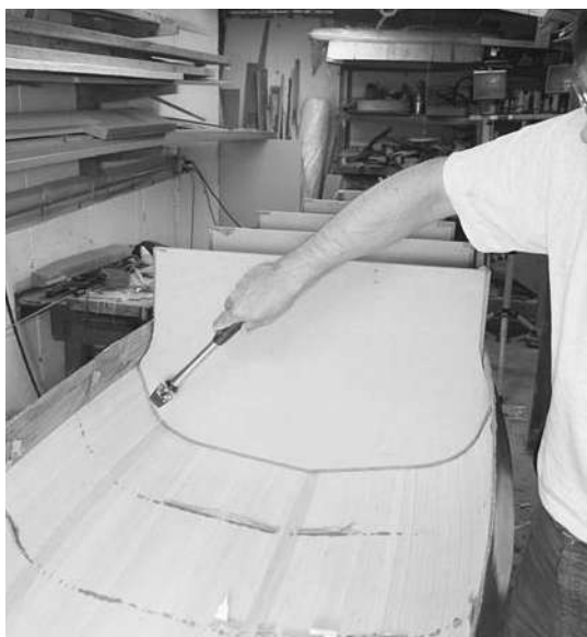
Figure 7-18. The staple holes will often wick a little epoxy onto the forms. This is why the forms have tape on the edges, but sometimes you may need a little persuasion to get the boat off. Some light raps with a hammer usually do the trick.
