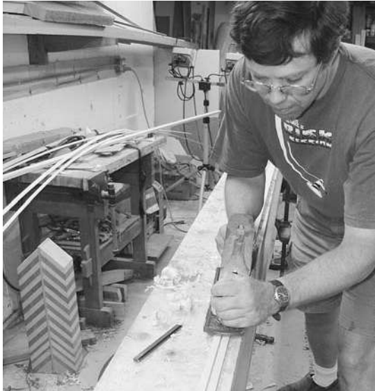
Figure 12-29. To save weight on the gunwales I used basswood and tapered them at each end. Place both gunwales side by side and plane them both simultaneously to assure they match.
