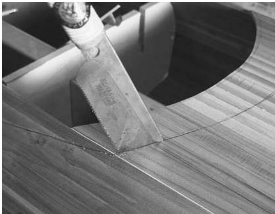
Figure 13-40. You can use a jigsaw to cut out the cockpit area, but it tends to cut a rough line. A Japanese saw makes a cleaner cut, but it does have a little trouble cutting a curve. I used the flexible tip of a Japanese “beading” saw to make the cut. Approach the feature line from both sides and avoid cutting too far.
