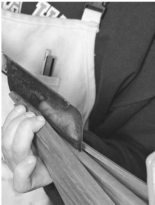
Figure 13-29. You start the deck much like the hull. This time match your rolling bevel to the bevel on the top strip of the hull. The ends of this design meet in a V-shape that requires a matching taper on the strips approaching from both sides. Rough this out with a plane and then fine-tune it by dragging a saw through the seam.
