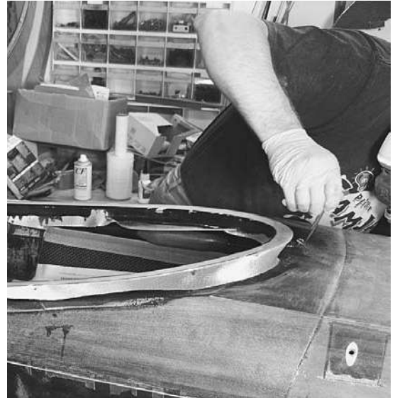
Figure 13-55. After the coaming lip is installed, trim off the excess riser above the lip with a coping saw, grind and sand the top smooth, and round over all the corners. The inside surface of the coaming riser is not glassed over yet, but you could have. Here I wrapped one piece of bias-cut 4-ounce cloth from under the deck, up the riser, over the top of the lip, and then down under the bottom side of the lip onto the outside of the coaming riser.
