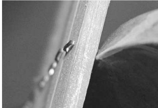
Figure 6-12. Since you will be pulling out the staples eventually, you do not want them pushed in flush with the strip. A little gap between the staple and the wood will provide a starting point for removing the staples later. If you do not bevel the forms, as in this example, you need staples long enough to reach across the gap. You can also align the staples near the close edge.
