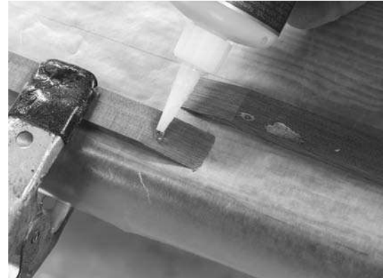
Figure 6-3. If you have the time, you can use carpenter's glue and a clamp to glue the scarf joint. Be sure the strips are aligned in a straight line; it is easy to have one end go off at a funky angle. For a quick joint, use CA glue. Spread glue on one surface, then spray the other with accelerant. Carefully align the ends and press the pieces together.
