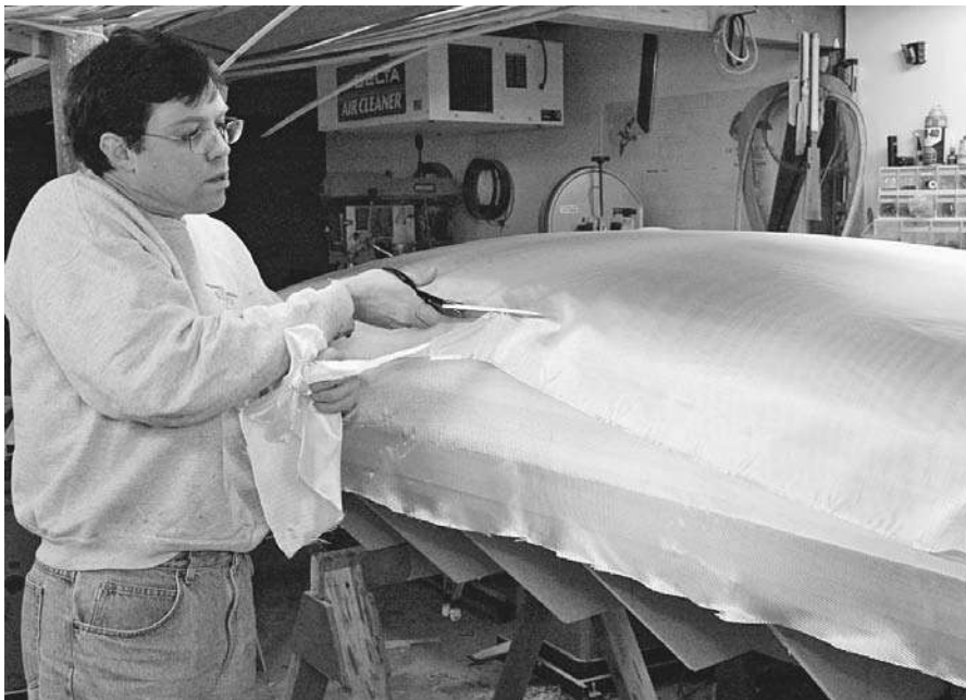
Figure 11-18. The Coot is too wide to span with one piece of cloth. For a light layup, you can overlap two layers along the centerline, but I wanted some added durability, so I overlapped two layers of 6-ounce cloth across the whole bottom. Trim the cloth so it follows the line of the strips. This helps hide any irregularity that may result.
