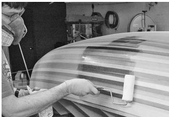
Figure 9-3. A seal coat limits how much epoxy is absorbed later when applying fiberglass. Brush on a little epoxy, then spread it around with a roller. There should be no need to thin the epoxy. The seal coat is not a requirement, but it does make the later coats that wet out the fiberglass a little bit easier to accomplish.
