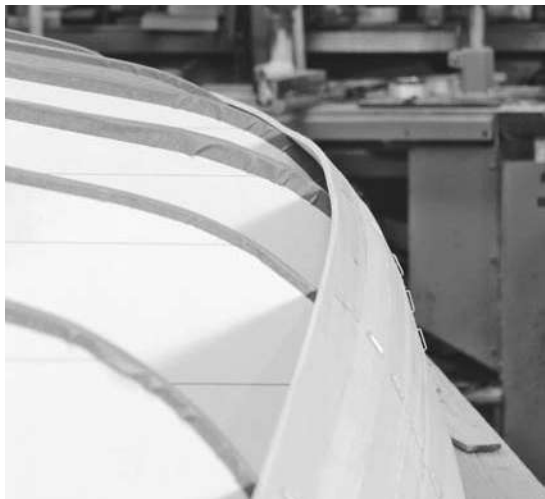
Figure 6-36. Watch your strips carefully as you install them. Bending them to make them conform to the curves can impose a lot of stress, particularly on short boats like the Nymph . This piece is starting to show some buckling as it turns the corner. Adding more strips probably won't make this go away. It is caused by trying to bend the strip the "hard" way across its width instead of the "easy" way across its thickness. Eventually the strip buckles to transfer the bend to the "easy" way.
