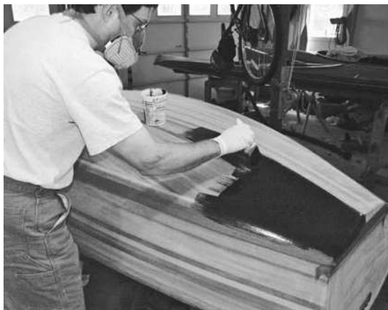
Figure 9-30. Mixing graphite powder into epoxy, creating a black paint, makes a low-friction surface that protects against scratches. Add about 10% to 15% powder by volume to the epoxy. Here I am applying it with a brush, but a roller also works well. The masking tape keeps the black stuff where I want it. Note that the finish will tend to make your clothes black if you rub against it.
