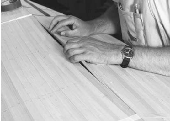
Figure 6-41. As you get toward the middle of the last strip, start fitting the other end. Make some alignment marks so you know where things should line up when it all fits together. As you work back toward the middle again, start working on getting the length right. By carefully checking the fit, noticing where the strip binds up, and gradually planing away at the high spots you should be able to make a snug-fitting strip. By pushing up on the existing strip from underneath you can open up the gap a bit while you press the new strip in place. Check the fit with the strip dry, and then add glue. Strips of strapping tape stretched across the boat will pull the seam tightly together.
