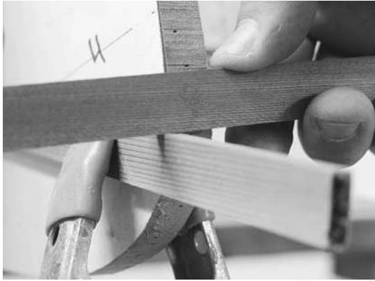
Figure 6-8. As you move down the length of the boat, check the gap at each form and plane it until it disappears. In between forms, roll your wrist as you plane to gradually transition between the bevels at each form. With a little practice, this whole process will only take a couple of minutes.
