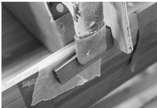
Figure 13-22. Butt together the strips cut with the miter box in place on the boat while stripping. Use waxed paper so the scrap strip used to help align the joint does not stick to the boat. Put masking tape on either side of the joint to hold the strips in place relative to the strip below.
